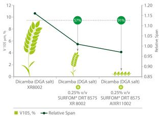
1% of commercial Dicambadialycolamine salt with 480 g/l of acid at 40 psi with wind speed of 8m/s, droplet size obtained with Sympatec HELOS lati Vario laser diffraction.
